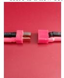
I modify the connector (at my/your own risk!) by drilling a pair of 1/16 holes in the ground side of the connector. Don't penetrate the copper pole:
